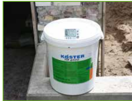
3. The hobcock contains both components and allows for mixing in the bucket (min. mix time 3 mins).
