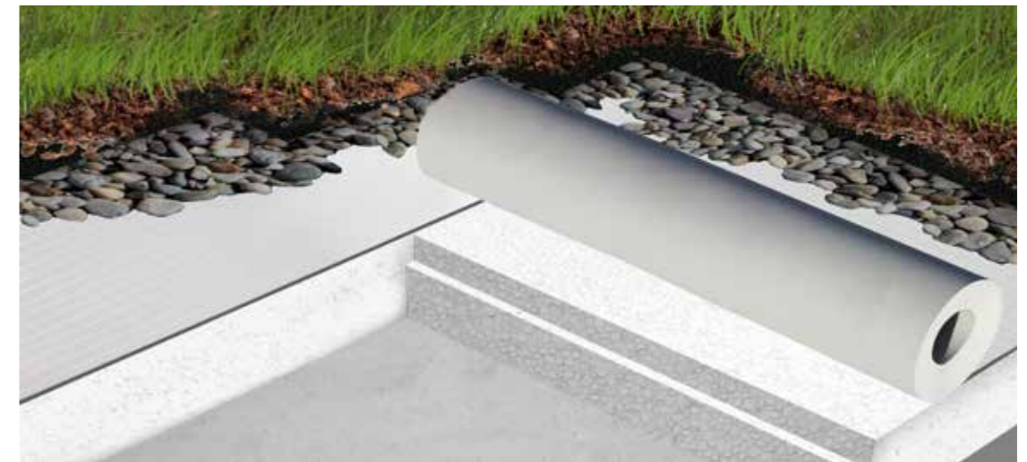
KÖSTER TPO membranes can be loose laid under green roofs where the green roof serves as a ballast and protects the membrane against wind uplift. Additionally, KÖSTER TPO Membranes are resistant to root and rhizome penetration. This allows for planting and cultivation directly on top of the membrane.
