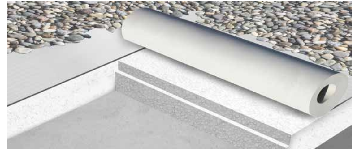
If the membrane will be covered with a ballast such as gravel, the membrane can be loosely laid. By loose laying the membrane with ballast, mechanical fastening is no longer required.
