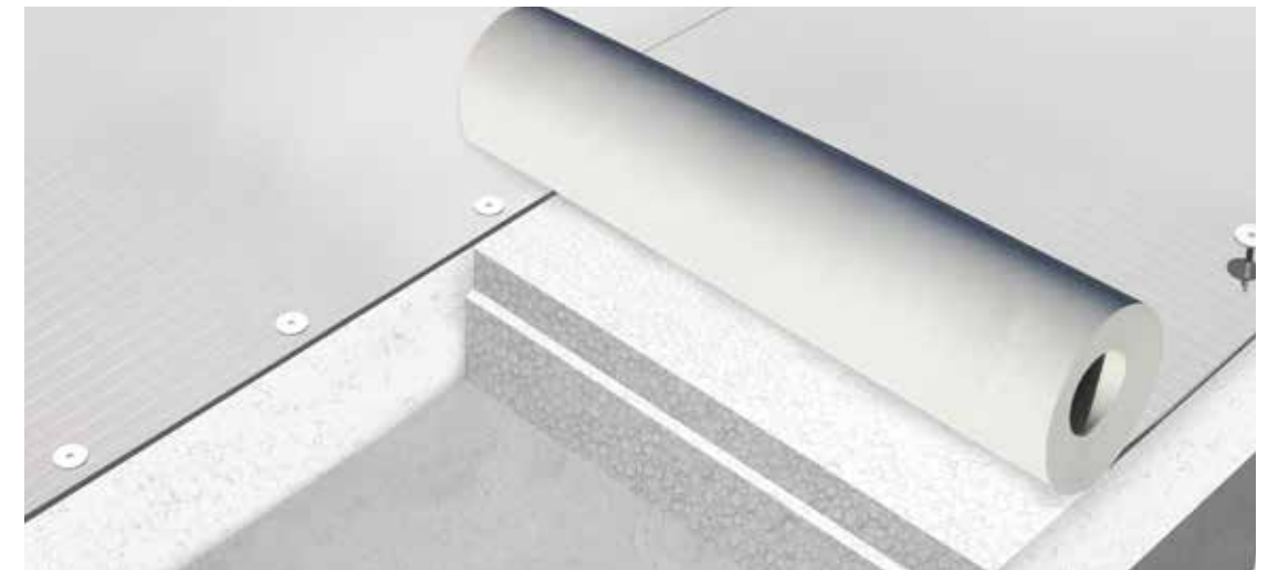
The KÖSTER TPO Membrane is mechanically fastened using disc anchors. The disc anchors are securely fixed through the insulation to the substructure (i.e. supporting construction). Upon request, KÖSTER can calculate the wind load in order to determine the number of fasteners required.
