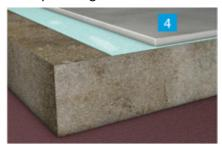
layer thickness of 2-8mm. It can be walked on after only 3 hours of curing time and it is abrasion and wear resistant. KÖSTER Self-Levelling Floor 15 is used for levelling out mineral substrates inside and outside, underneath tiles, ceramic coverings, screeds - also for wet rooms, balconies and terraces. KÖSTER Self-Levelling Floor 15 is not a decorative final coating.
