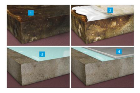
KÖSTER ORS is an oil-removal and containment treatment process to rehabilitate concrete surfaces making them suitable to receive any type of flooring system. The KÖSTER Oil Removal System (ORS) consists of two components:
