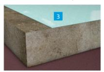
very low viscosity and can therefore be applied with a roller. A spread rate of about 0.4 liters per square meter is required for the KÖSTER ORS-C. After a curing time of about 15-20 minutes silica sand is broadcasted into the still wet coating. A spread rate of 0.5 kg of sand (mesh size 0.3-0.7 mm) per square meter is required. The sand is important for the adhesion properties regarding the subsequent coatings. After
